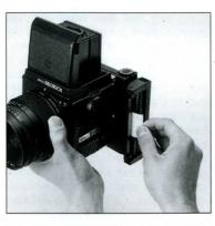
A. 撮影がすみましたら、右側に白 タブがくるように左手でカメラを持 ち、右手の親指と人さし指で白タブ をつまみます。 A. Upon taking the picture, hold the camera with the left hand so that the white tab can be pulled with the right hand, as illustrated. Then, grip the white tab firmly with the right thumb and forefinger.
